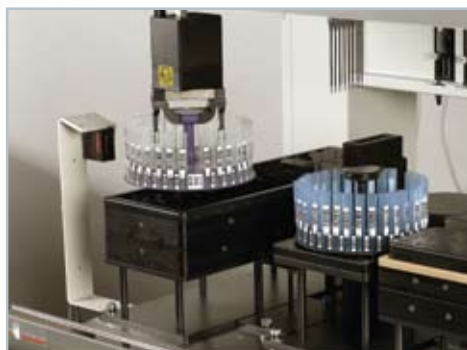
On-deck MCLs with Fly-By Bar Code Reader for cocktails prepared in individual sample tubes
