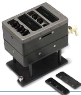
Rack for 56 IOTest reagent vials with covers on top of a TEU. (Covers of the first 7 rows were removed to show the tilted vials.)
